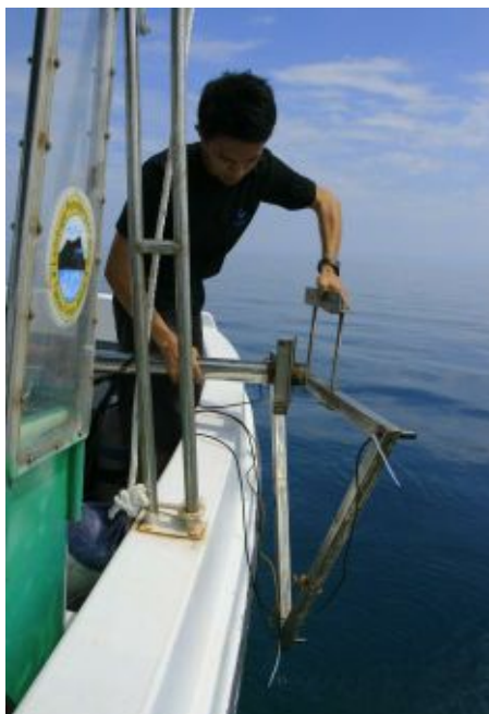
Figure 7 (left). Hydrophone frame being clamped onto a horizontal plate welded onto the bottom end of the pole
