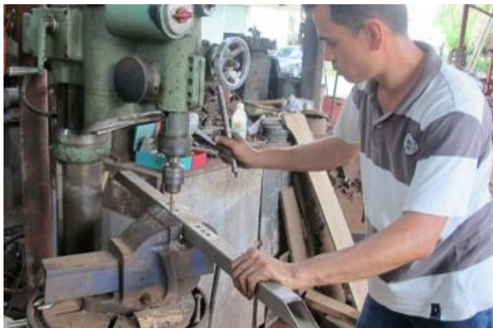
Figure 2. Drilling holes for the clamp
