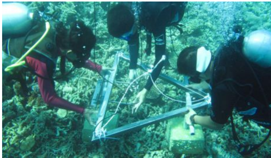
Figure 6. Attaching the acoustic frame to the concrete blocks
