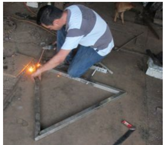
Figure 3. Welding the frame
