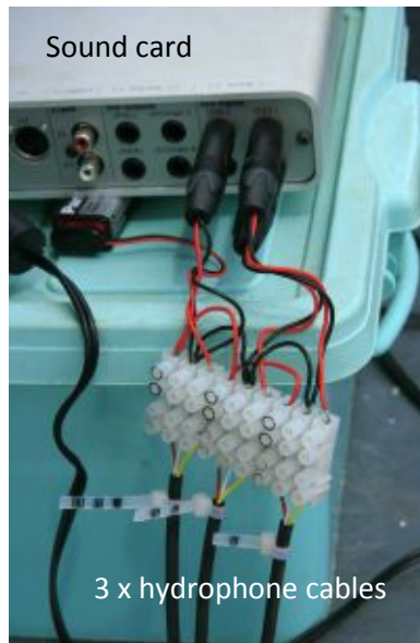
Figure 11. Hydrophone cables Attached tote sound card
